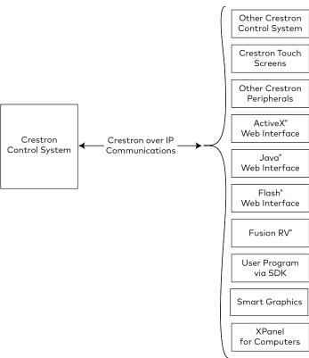
Multiple listeners can be added to the Crestron control system via the user program. Crestron recommends performing a security scan on the control system without a program and then performing the scan again with a program. This will help identify whether any security breaches are created by loading the program.
