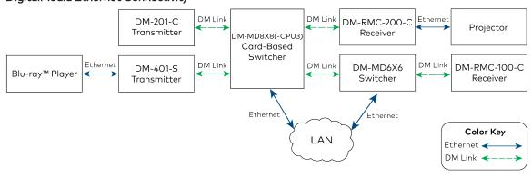
The main Ethernet uplink to a DM system occurs at the DigitalMedia switcher.
