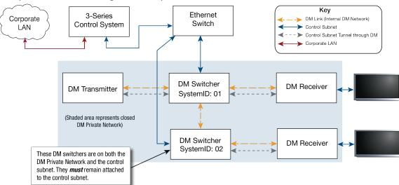
**NOTE:** The SystemID can range from 01 to 64 and must be unique for each DM switcher. By default, the SystemID is set to 01. The ID can be set via the front panel, the SIMPL program, or the System Info tool in Crestron Toolbox. Each DM switcher must be directly connected to the corporate LAN. One DM switcher cannot receive Ethernet via another DM switcher, and each DM switcher must receive an IP address from the control subnet.
