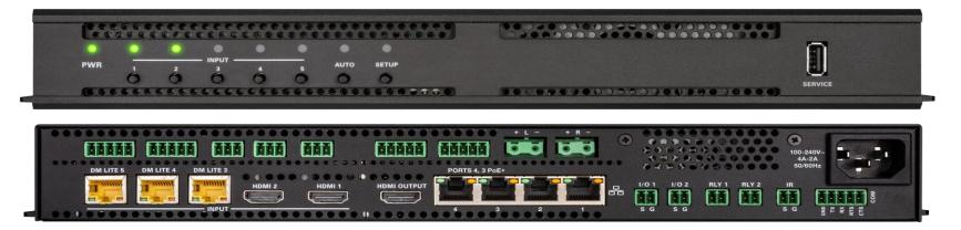
Plus a 4-port Gigabit Ethernet switch with two PoE+ ports.
